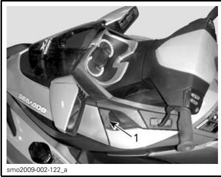
smo2009-002-122_a TYPICAL - STORAGE BIN ACCESS 1. Front cover latch handles (one each side)
