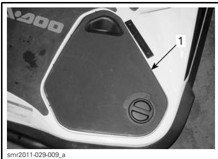
1. Starboard access panel
