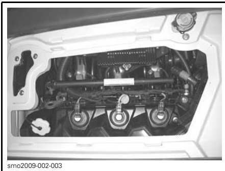
VENTILATION BOX REMOVED
