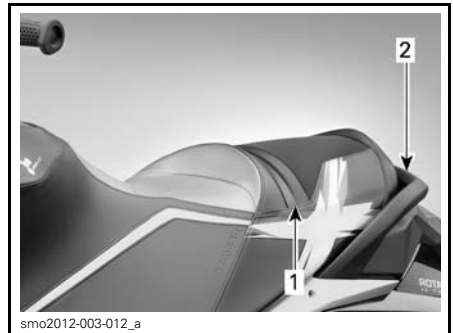
TYPICAL - PASSENGER HANDHOLDS
