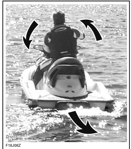
TYPICAL - STEERING DIRECTION REVERSED WHEN BACKING
