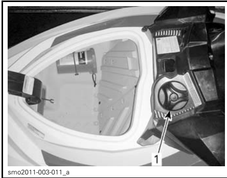
TYPICAL - FUEL TANK CAP LOCATION
