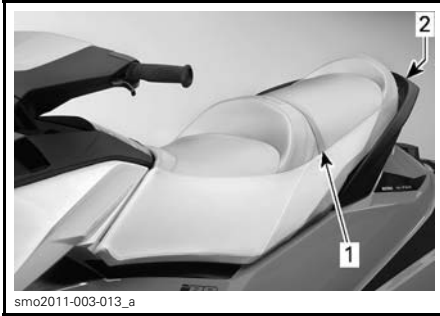
TYPICAL - PASSENGER HANDHOLDS
