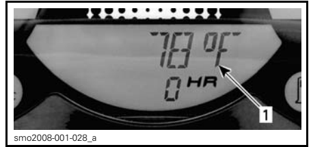
TYPICAL 1. Water temperature
