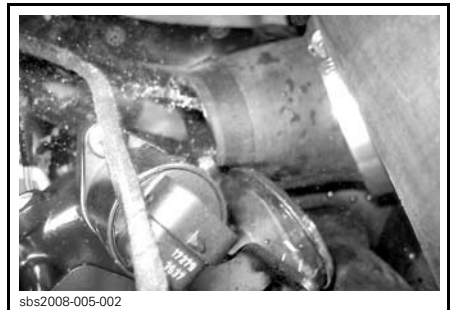
WATER EXPELLED FROM INTERCOOLER
