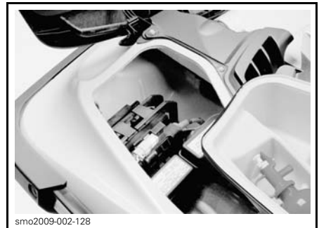
BATTERY AND FUSE ACCESS - RH STORAGE BIN REMOVED
