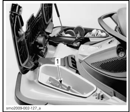
1. Fire extinguisher holder location
