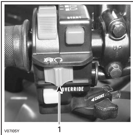
TYPICAL 1. Engine stop switch
