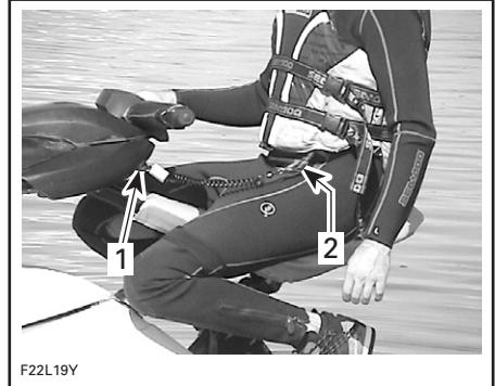
1. Safety lanyard cap on the post 2. Safety lanyard secured on operator's PFD
