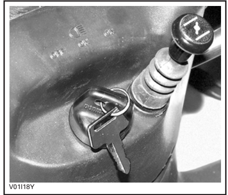
CHOKE LEVER IN THE FULL CHOKE POSITION
