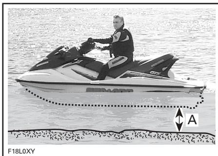
1. *Maintain at least 90 cm (3 ft) underneath the lowest rear portion of the hull when all passengers are aboard*
