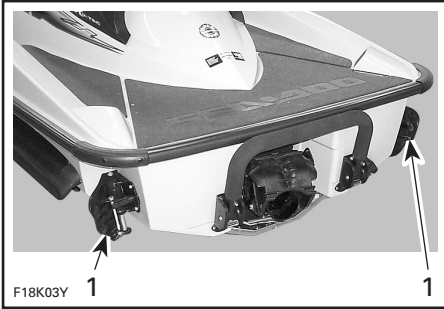
1. Side vanes turn following steering movement
