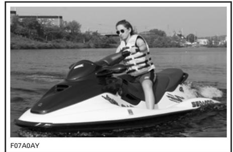
Turning the handlebar pivots the jet pump nozzle which controls the watercraft direction. Turning the handlebar to the right will turn the watercraft to the right and inversely. The throttle should be applied to turn the watercraft.
