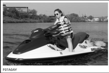
Turning the handlebar pivots the jet pump nozzle which controls the watercraft direction. Turning the handlebar to the right will turn the watercraft to the right and inversely. The throttle should be applied to turn the watercraft.
