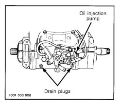
With spark plugs in place, crank engine to drain crankcase. Reinstall crankcase drain plugs.
