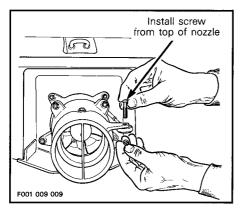
WARNING: Steering cable ball joint must be adjusted, if not possible damage could occur to either nozzle or venturi when turning the handlebar. Also steering cable could possibly break causing a lost of directional control.
