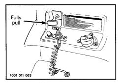
Firmly grip handlebar and place both feet on the floorboard. Depress the starting button.
