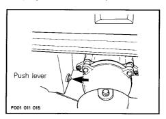
WARNING: Always make sure bilge drain plug is properly installed in the drain hole and lever is safely locked.
