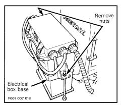
2- Remove electrical box ass'y from top of battery.
