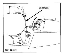
The dipstick indicates the amount of oil to be added in the reservoir. Oil level should be maintained between FULL and ADD marks. Before checking oil level, have the watercraft leveled, then wipe the dipstick and insert it in the reservoir neck. Do not screw cap. Remove dipstick and read the level.
