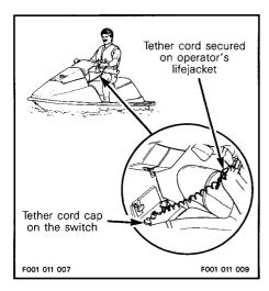
WARNING: Should the engine be stopped, watercraft directional control will not be available. To prevent theft or unauthorized use, remove the tether cord from switch.
