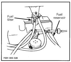
Before opening fuel filter, hold the bowl in a dry rag and proceed carefully to avoid fuel spillage.
