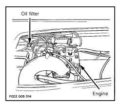
Visually inspect the oil filter at least once a month. Ensure that it is free of water, clean and no foreign particles are present, if so, refer to an authorized dealer for replacement.
