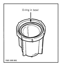
Install filter bowl and firmly hand tighten.
