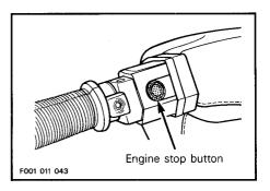
WARNING: When the engine is stopped, watercraft directional control will not be available.
