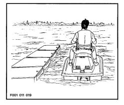
CAUTION: The engine should be started with at least 60 cm (2 ft) of water below the hull.
