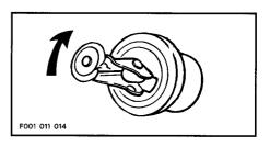
Reinstall bilge drain plug and fully push the plug lever to locked position.
