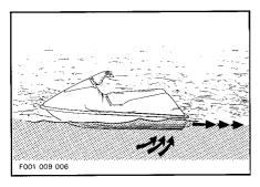
WARNING: It is important to keep in mind that as soon as the engine is running, the jet pump is constantly producing a thrust causing the watercraft to move forward. Therefore, whenever the engine is to be started, the operator should always be sitting on the watercraft.
