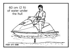
CAUTION: The engine must be shut off before less than 60 cm (2 ft) of water is underneath the hull. Shells, sand, pebbles or other objects could be drawn up by the jet pump and damage impeller, components or clog or jam cooling system.
