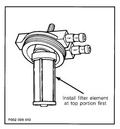
Inspect O-ring for damage, replace if necessary. Ensure the O-ring is well positioned into recess of filter bowl.
