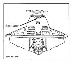
Pull latch lever to insert it over the rear hook. Release latch lever then firmly push on rear of the seat to relatch.
