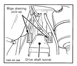
This watercraft features a vacuum activated syphon. Two pick-ups use a low pressure area in the jet pump to syphon the water out of the bilge.
