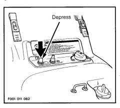
NOTE: Engine will not run if the tether cord is removed.
