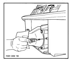
Secure jet pump nozzle to ball joint. Make sure to install screw from top of nozzle as shown. Tighten nut to 10 N•m (7 lbf•ft).
