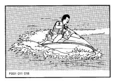
Turning the handlebar pivots the jet pump nozzle which controls the watercraft direction. Turning the handlebar to the right will turn the watercraft to the right and inversely. However, the throttle must be applied to turn the watercraft.
