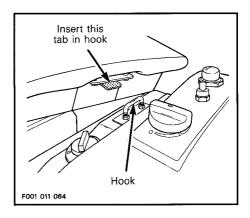
When reinstalling the seat, insert seat front tab into body hook.
