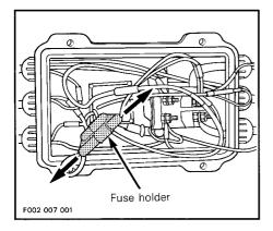
Replace the fuse by one of the same rating. Ensure to install the fuse in compartment where a wire is located. Align wires when closing fuse holder. Make sure to properly close the fuse holder.
