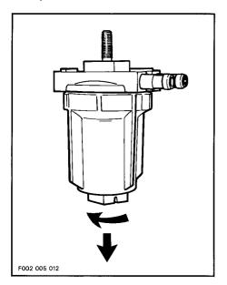
Pull the filter element toward the bottom.
