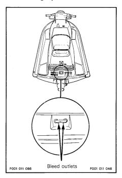
When engine is running, water must flow from these holes. This allows air in tuned pipe and in engine water jacket to escape. CAUTION: Should water not flow from these outlets a few seconds after engine starts, immediately stop engine and refer to an authorized dealer for servicing.
