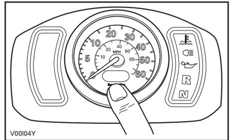
Press once to switch from odometer to tripmeter or vice versa. Press and hold to reset while in trip meter selection.
