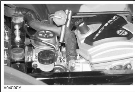
Fill the radiator until the coolant comes out by the thermostat housing hole. Install the bleeding screw then remove the hose pincher.
