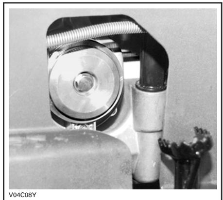
Remove the oil filter and replace with a new filter.
