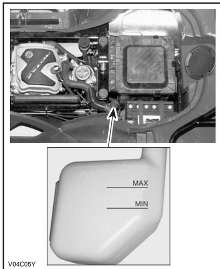
With vehicle on a level surface, liquid should be between MIN. and MAX. level marks of coolant reservoir.
