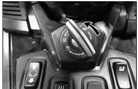
KEY POSITION TO OPEN FRONT STORAGE COMPARTMENT
