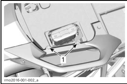
1. 2 plastic rivets under the seat
