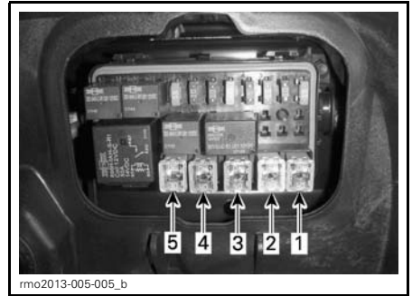
JCASE FUSES - LEFT FUSE BOX
