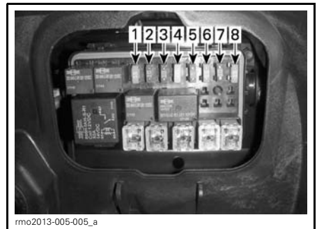
FUSES - LEFT FUSE BOX
