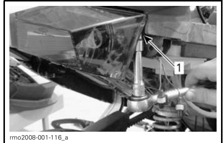
1. Removing Torx screw behind lens
