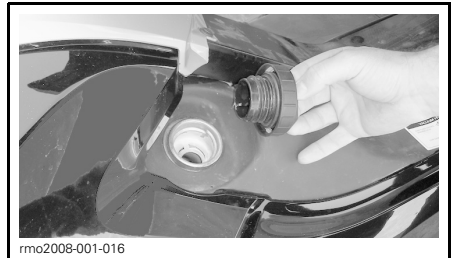
FUEL CAP ON LEFT SIDE UNDERNEATH SEAT
