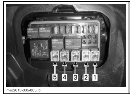
JCASE FUSES - LEFT FUSE BOX
