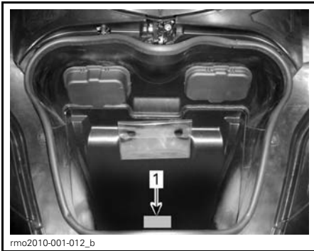
1. Label 3 located in the front storage compartment
