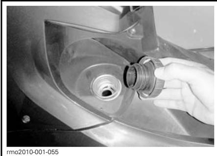
**BOUCHON DE RÉSERVOIR D'ESSENCE DU CÔTÉ GAUCHE SOUS LE SIÈGE**
