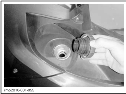
FUEL CAP ON LEFT SIDE UNDERNEATH SEAT
