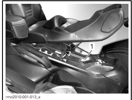
1. Fuse box located under the seat
