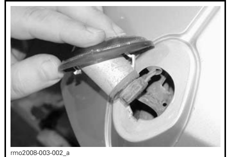
3. Turn the bulb holder clockwise and remove it from the connector.
