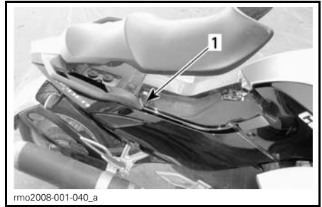
1. Fuse box located under the seat
