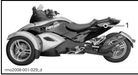
1. Battery located behind the rear left side panel
