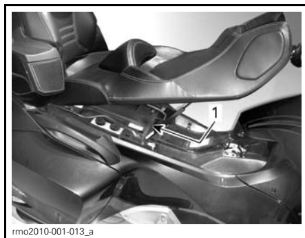
1. Fuse box located under the seat
