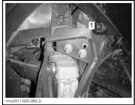
RIGHT SIDE SHOWN 1. Adjust through this hole
