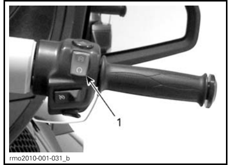
1. Engine stop switch
