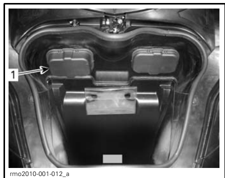
1. Fuse box in front storage compartment
