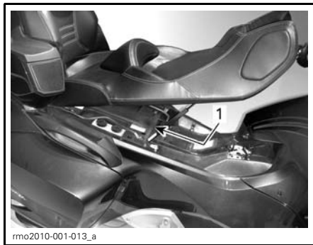
1. Fuse box located under the seat
