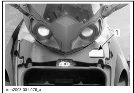
1. Fuse box located under the service cover behind the front storage compartment
