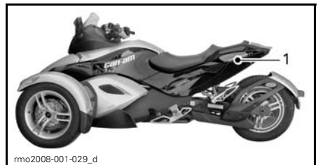
1. Battery located behind the rear left side panel
