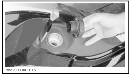
FUEL CAP ON LEFT SIDE UNDERNEATH SEAT
