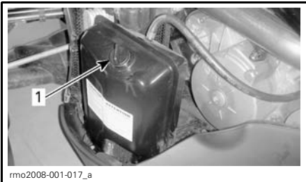
1. Oil tank and dipstick
