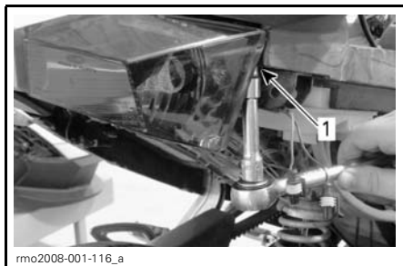
1. Removing Torx screw behind lens
