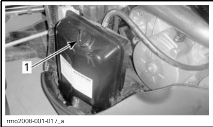
1. Oil tank and dipstick
