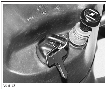
CHOKE KNOB LEVER IN THE OFF POSITION
