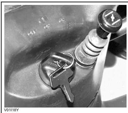
CHOKE LEVER IN THE FULL CHOKE POSITION
