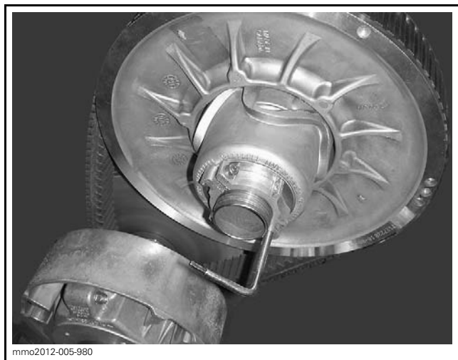
TYPICAL - PULLEY EXPANDER INSTALLED ON ADJUSTER HUB
