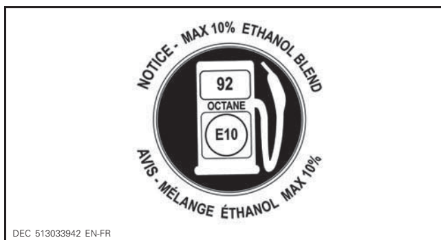
ON FUEL CAP - ON 600 EFI ENGINE IN COUNTRIES USING RON OCTANE RATINGS
