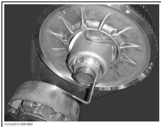
TYPICAL - PULLEY EXPANDER INSTALLED ON ADJUSTER HUB
