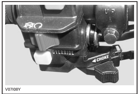
CHOKE LEVER IN THE OFF POSITION
