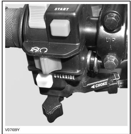
CHOKE LEVER IN THE FULL CHOKE POSITION
