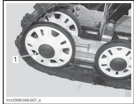
1. Deflection O-ring aligned with slider shoe
