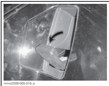
PULL TO ENGAGE REVERSE GEAR
