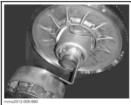
TYPICAL - PULLEY EXPANDER INSTALLED ON ADJUSTER HUB
