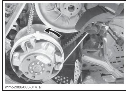
6. Pull the rope using a sharp, crisp pull so the rope comes free of the drive pulley.
