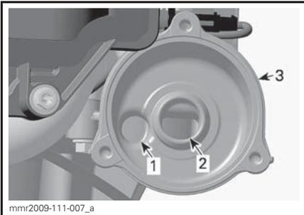
1. Oil inlet orifice from the oil pressure pump
