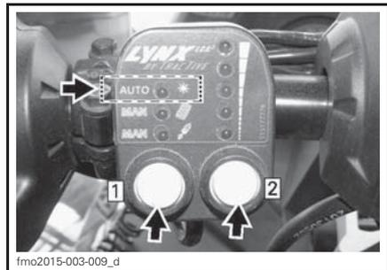
To use preselected values push the left button till AUTO led lights up. Push the right knob to set the preselected spring preload and damping force. Upwards
