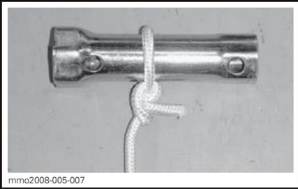
3. Attach the other end of emergency rope to the starter clip supplied in the tool kit.
