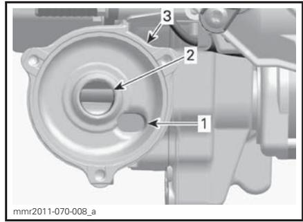
1. Oil inlet orifice from the oil pressure pump
