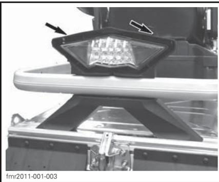
**NOTICE** Plastic retaining pins may break if taillight assembly is forced sideways. Avoid sideways movement when pulling taillight out.
