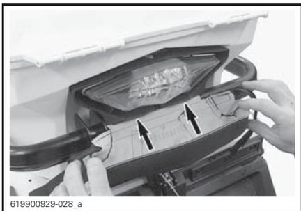
2. Pass the retaining straps behind the taillight.
