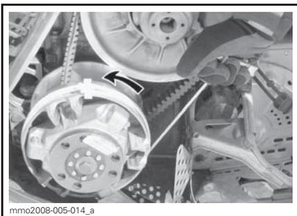
6. Pull the rope using a sharp, crisp pull so the rope comes free of the drive pulley.
