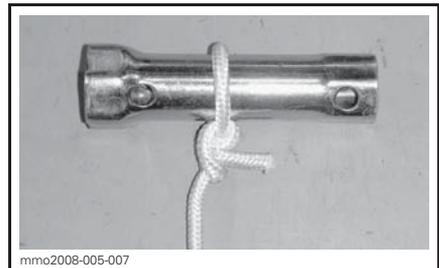
3. Attach the other end of emergency rope to the starter clip supplied in the tool kit.
