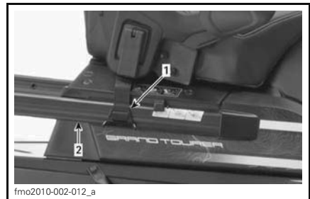
1. Retaining strap 2. Rear bumper
