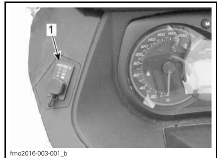
1. Battery Display/Charging plug
