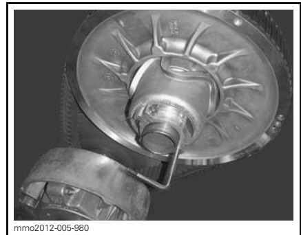
PULLEY EXPANDER INSTALLED ON ADJUSTER HUB
