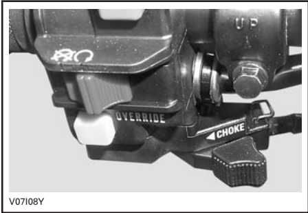
CHOKER LEVER IN THE OFF POSITION
