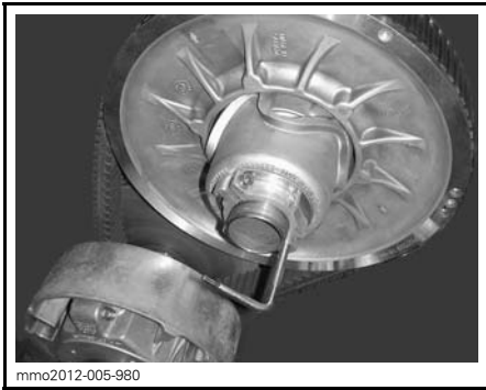
PULLEY EXPANDER INSTALLED ON ADJUSTER HUB
