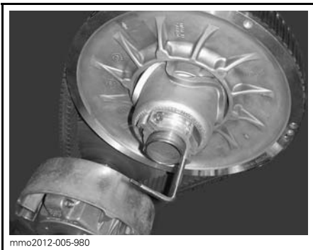
PULLEY EXPANDER INSTALLED ON ADJUSTER HUB
