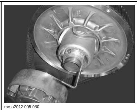
PULLEY EXPANDER ON ALUMINUM ADJUSTER HUB
