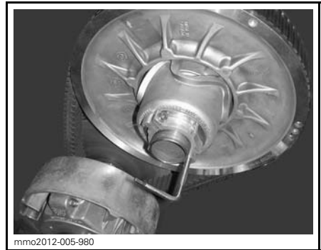
PULLEY EXPANDER INSTALLED ON ADJUSTER HUB
