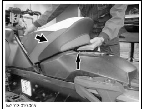
**NOTICE** Pull the handle upwards when removing the seat.
