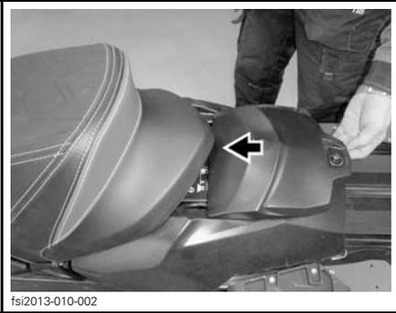
Finish the installation by locking the battery cover.
