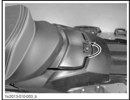
Remove the seat by pulling and lifting at the same time.
