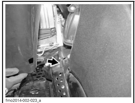
To remove a side panel, open it then lift it up. Free the lower hinge from its slot, then free the upper hinge by lowering the panel.
