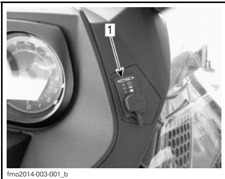
1. Battery Display/Charging plug
