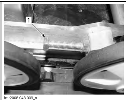
1. RH adjustment screw
