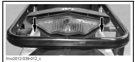
TYPICAL - CAREFULLY PULL OUT AT CORNERS
