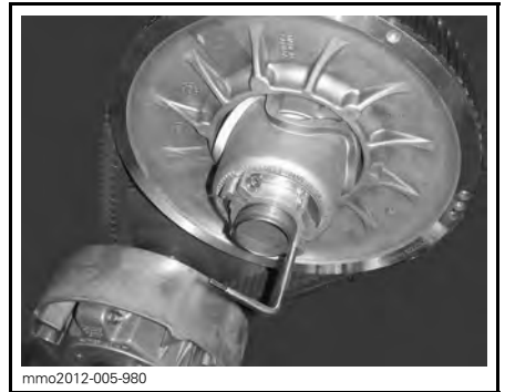
PULLEY EXPANDER INSTALLED ON ADJUSTER HUB
