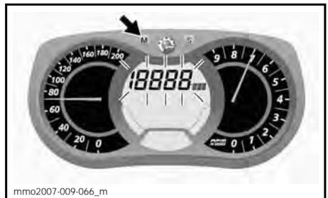
While display is flashing, press SET (S) button to select RPM mode.
